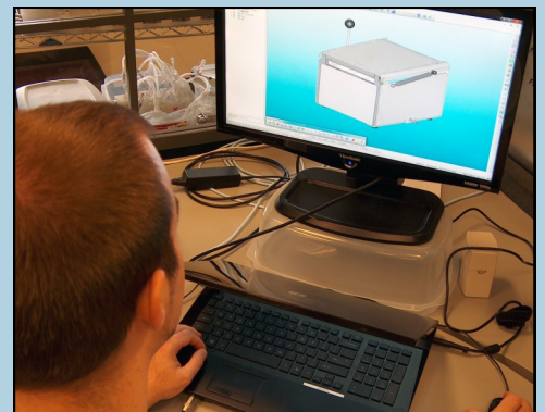
Andrew Shepardson uses Creo Elements/Direct to design MEC's proprietary Universal Electro-Mechanical Interface Fixture for functional test of early prototypes, proto/pilot units and low-medium volume production electronic assemblies.
